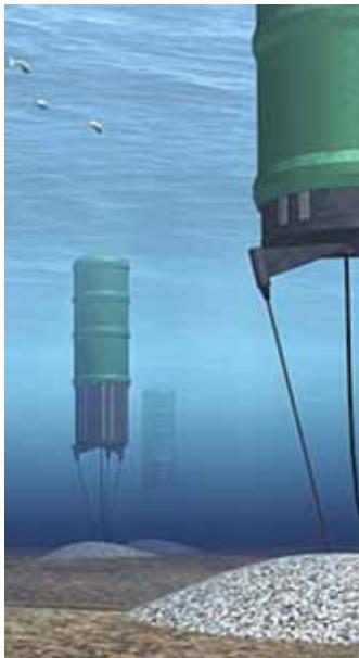
Figure 7: The Archimedes Wave Swing [AWS, n.d.].
