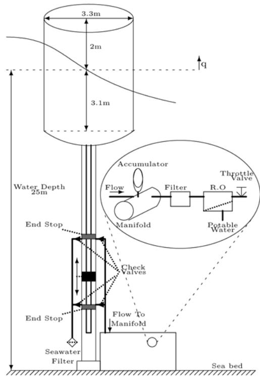
Figure 11: Conceptual diagram of a heaving buoy wave energy converter.
