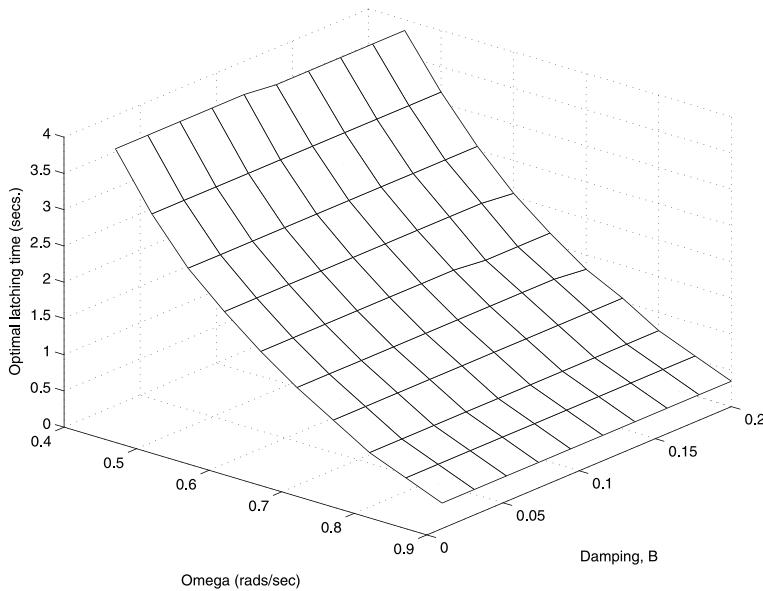
Figure 14: Variations in  $T_L^{opt}$  with B and  $W_w$ .
