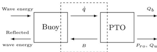
Figure 15: Coupling between buoy and PTO system.
