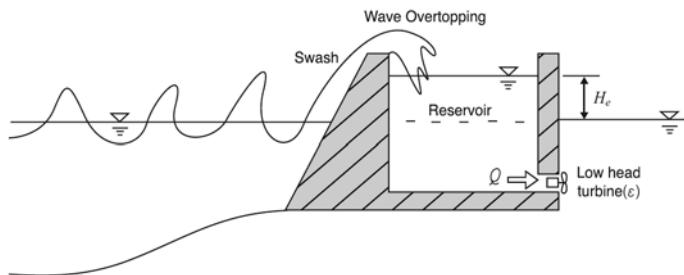
Figure 10: The principle of overtopping.
